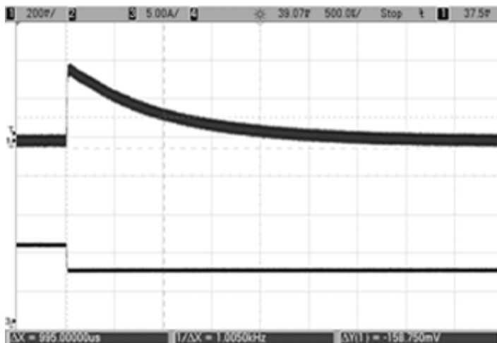
Step Load Transient Response (Vin = 48V, Vout = nom, Cload = 1μF || 10μF, Iout = 50 to 75 to 50% of full load, Ta = +25°C) Ch1 = Vout, Ch2 = Iout.
