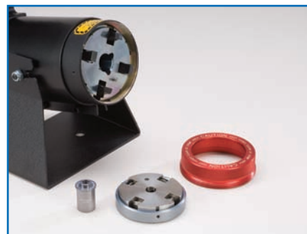
3. Pull out the Locator by hand.
