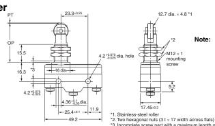
Note: Do not use the M12 mounting screw and the case mounting hole at the same time, or the case may be damaged.
