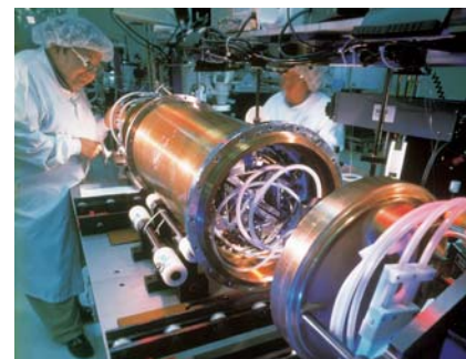
Telecommunications Undersea Cable Repeater
