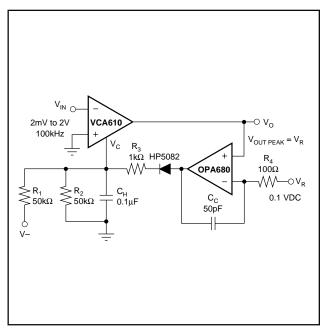
FIGURE 7. This AGC Circuit Maintains a Constant Output Amplitude for a 1000:1 Input Range.
