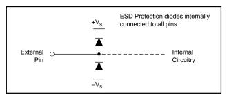
FIGURE 4. Internal ESD Protection.
