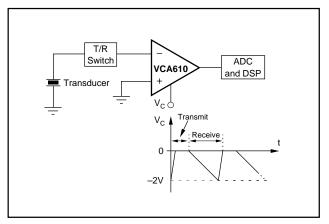
FIGURE 5. Typical Ultrasound Application.
