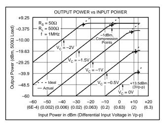
FIGURE 2. Input and Output Range.
