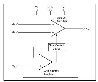
FIGURE 1. Block Diagram of the VCA610.
