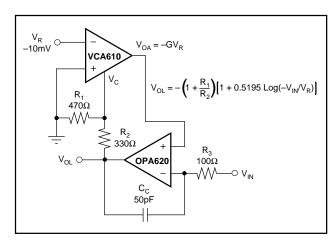
FIGURE 9. Driving the Gain Control Pin of the VCA610 with a Feedback Amplifier Produces a Temperature-Compensated Log Response.
