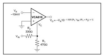
FIGURE 10. Signal Drive of the VCA610 Gain Control Pin Produces an Exponential Response, Re-expanding Signal Companded by Figure 9.
