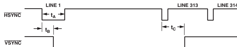
Figure 20. Timing Register 1 in PAL Mode
