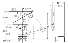
Adjustable Roller Lever, Form Lock (with Metal Lever, Rubber Roller) (D4N-□□2H) (Reference Values)
