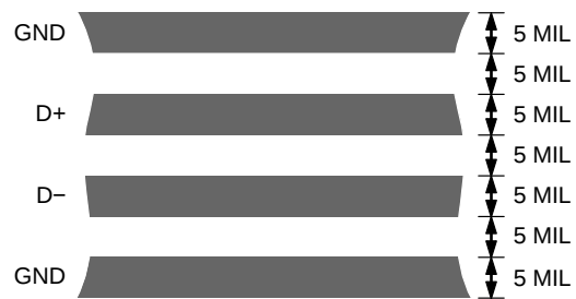
Figure 22. Typical Arrangement of Signal Tracks
