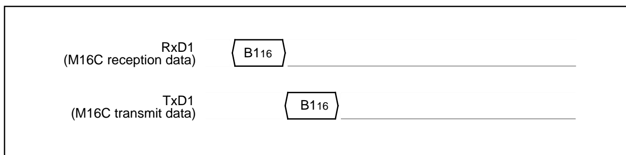
Figure 1.32.39. Timing of baud rate 19200
