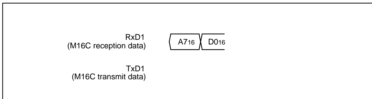
Figure 1.32.27. Timing for erasing all unlocked blocks
