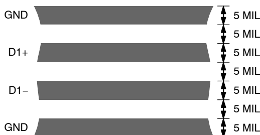
Figure 17. Arrangement of Signal Tracks
