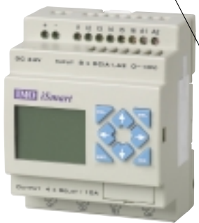
10 I/O (AC models), 12 I/O (DC models)
