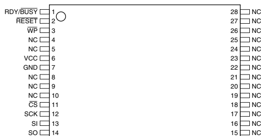
Figure 2-2. CASON – Top View through Package
