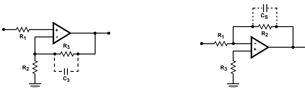
FIGURE 3. SUGGESTED OFFSET VOLTAGE ADJUSTMENT
