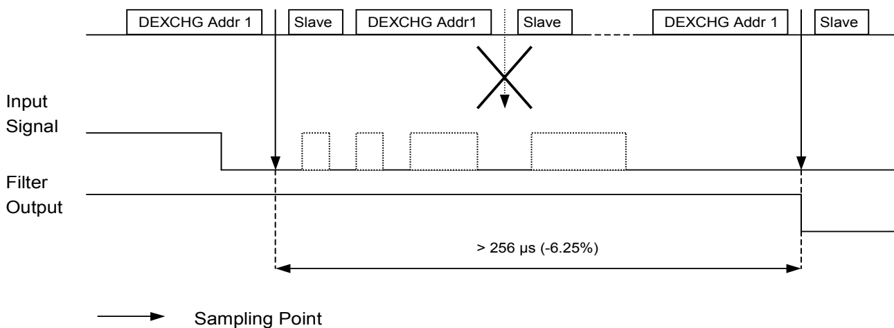
Figure 8: Principle of Delay Mode input filtering (exemplary for Slave with Address 1)
