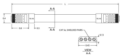
$Replace \textit{``XXX''} with \ length \ in \ Inches. \ Specify \ quantity \ of \ connectors \ to \ be \ installed --one, two \ or \ none.$
