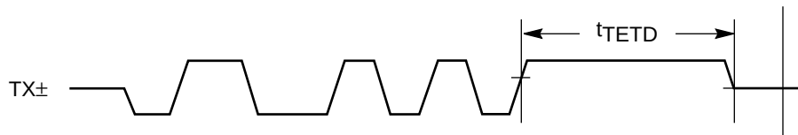
Figure 55 10 Mbps Transmit ( TX_{\pm} ) Timing Diagram
