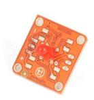
The **LED** is possibly the simplest actuator available. It's a low power light source available in many colors. It lights up when powered from an Arduino pin.
