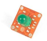
This module is an **ACTUATOR** therefore the connector is an INPUT that need to be connected to one of the **OUTPUT** connectors on the **TinkerKit Shield**.
