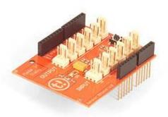
**Module description**: A green LED signals that the shield is correctly powered, a standard 6mm pushbutton allows you to RESET the board.
