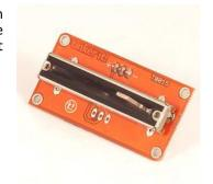
**Output**: This module outputs 5v when the slider is at one end and 0v when moved in the opposite way. When connected to an input on the Arduino using the TinkerKit Shield, you can expect to read values going from 0 to 1023.
