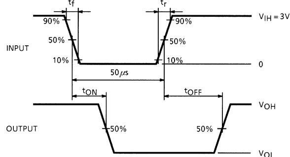
Note 1: Pulse Width 50  $\mu$ s, Duty Cycle 10%
