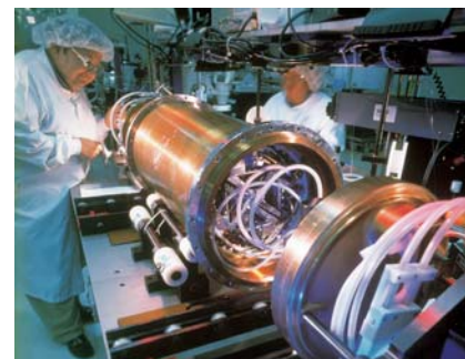
Telecommunications Undersea Cable Repeater
