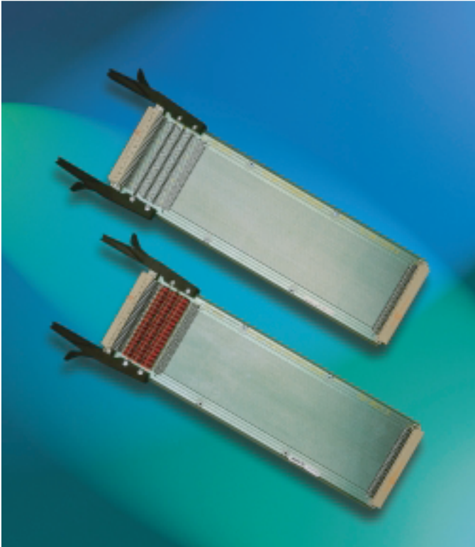
Standard and Super PTH extender boards
