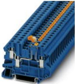
Knife disconnect terminal block, Connection type: Screw connection, Cross section: 0.14 mm<sup>2</sup> - 6 mm<sup>2</sup>, AWG: 26 - 10, Nominal current: 20 A, Nominal voltage: 500 V, Length: 65.4 mm, Width: 6.2 mm, Color: blue, Assembly: NS 35/7,5, NS 35/15
