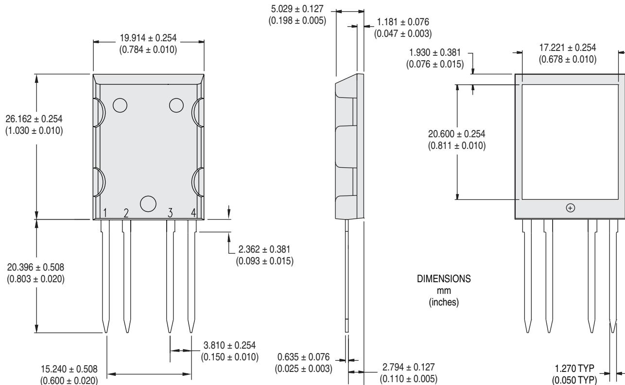
NOTE: Back-side heat sink meets  $2500V_{\text{rms}}$  isolation to the pins.
