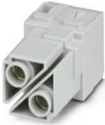
Contact insert module, number of positions: 2, power contacts: 2, control contacts: 0, Socket, Axial screw connection, 1000 V, 100 A, 10 mm<sup>2</sup> ... 35 mm<sup>2</sup>, application: Power
