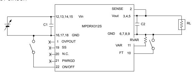
$\begin{array}{ll} \text{C1: } 100\mu\text{F} \, / \, 10\text{V} & \text{Ceramic Capacitor} \\ \text{C2: } 100\mu\text{F} \, / \, 6.3\text{V} & \text{Ceramic Capacitor} \end{array}$
