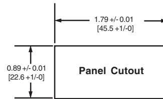
The mounting clip accommodates panel thicknesses up to 1/4" [6.4mm].
