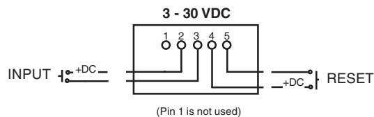
Terminal block will accept wire sizes from 14 to 24AWG.
