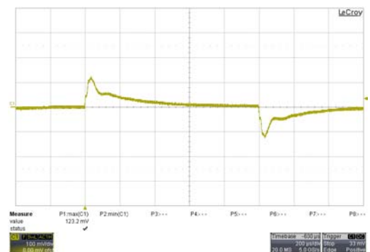
Transient Response to Dynamic Load Change from 100% to 75% of Full
