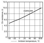
2.-(2) On resistance vs. ambient temperature characteristics
