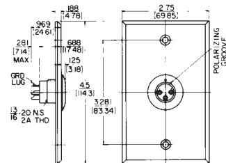
Wall plate with one B3M or B4M male receptacle mounted (in "D"-shaped hole to prevent turning) on standard single electrical outlet box. Cover mounting screws included.
