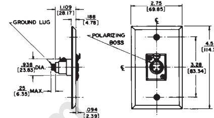
Wall plate with one, D3F or D4F female receptacle. Mounts on standard single electrical outlet box. Cover mounting screws included.
