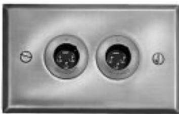
Wall plate with two, B3M or B4M male receptacles mounted (in "D"-shaped holes to prevent turning) on standard single electrical outlet box. Cover mounting screws included.
