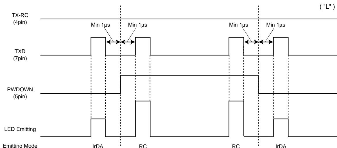
\*If TX-RC or TXD input pulse width is wider than 48μs, output LED emitting pulse will be turn off approximately 48μs.
