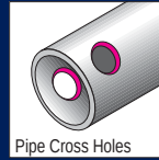
Pipe Cross Holes
