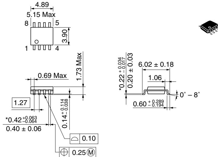
\*Dimension including the plating thickness
