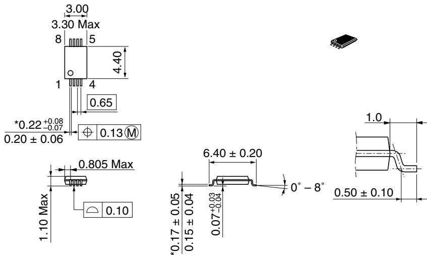
\*Dimension including the plating thickness
