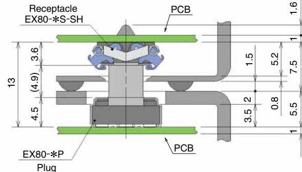
Note: The stacking length between boards of this connector is 13 mm.
