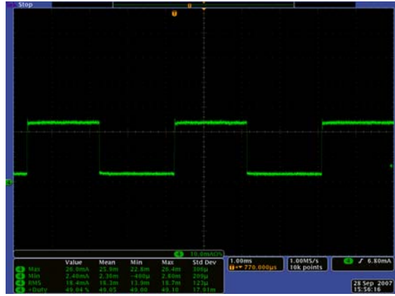
FIGURE 12. I_{LED} AT 50% PWM DIMMING (54 LEDs, 20mA, V_{IN} = 12V )
