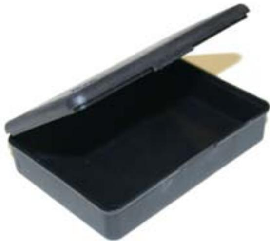
These boxes are made of conductive polypropylene with a surface resistivity of approximately  $5 \times 10^3$  ohm per square and a volume resistivity of about  $10^4$  ohm cm providing an excellent shield against electrostatic fields as defined in IEC 61340-5. They are suitable for primary packaging of electrostatic sensitive devices that do not have a built-in power source.
