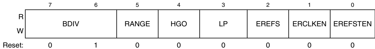
Figure 8-4. ICS Control Register 2 (ICSC2)
