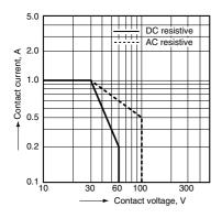
4. Electrical life Tested sample: HY1-12V, 6 pcs. Condition: 1 A 30 V DC resistive load, 30 cpm
