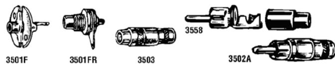
Type 3501FP for front panel mount in 0.25" (6.35 mm) holes in panels up to 0.125" thick. Type 3501FR for rear panel mount in 0.375" hole in panels up to 0.203" thick. Type 3502 has unique cable clamp with 0.406" O.D. shielded removable handle. Type 3503 extension jack has shielded removable handle 0.406" O.D. with cable clamp. Series 3558 are phone plugs with cable clamp and "snap-on" color-coded plastic handles in red, black, and white.
