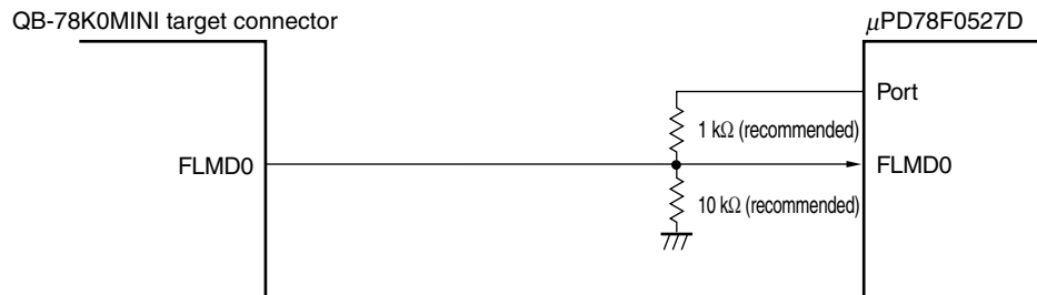
Figure 27-3. Connection of FLMD0 Pin for Self Programming by Means of On-Chip Debugging
