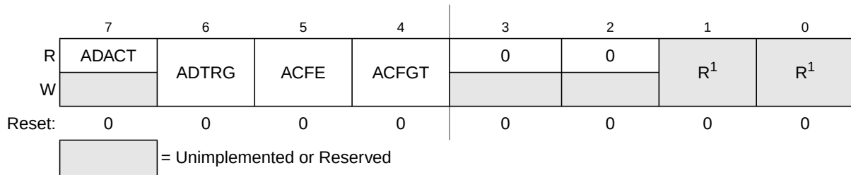
Figure 9-4. Status and Control Register 2 (ADCSC2)
