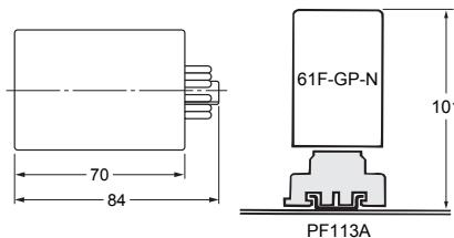
When mounting a Display Unit to a PF113A Surface-mounting Socket, secure the PF113A with the groove facing toward the bottom and then connect the 61F-GP-N the PFC-N8 accessory.
