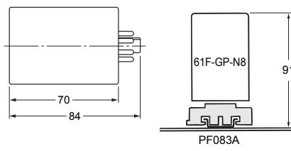
Use a PFC-N8 Mounting Bracket to mount the Level Controller to a PF083A Rail-mounted Socket.
