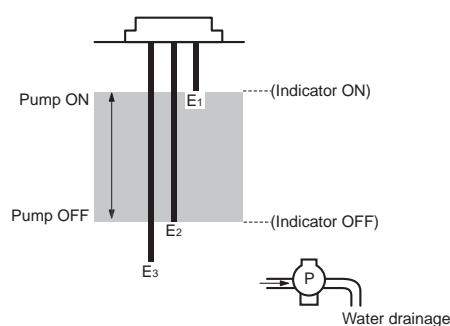
The pump starts when the water level reaches E<sub>1</sub> (indicator ON) and stops when the water level drops below E<sub>2</sub> (indicator OFF).
