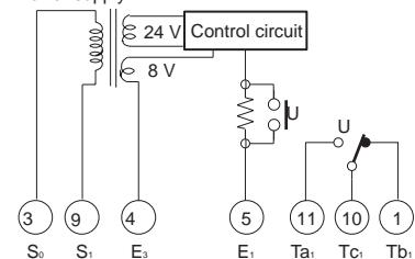
**Note:** When applying a self-holding circuit, short between terminals 5 and 6 and use terminal 7 as E<sub>2</sub>.
