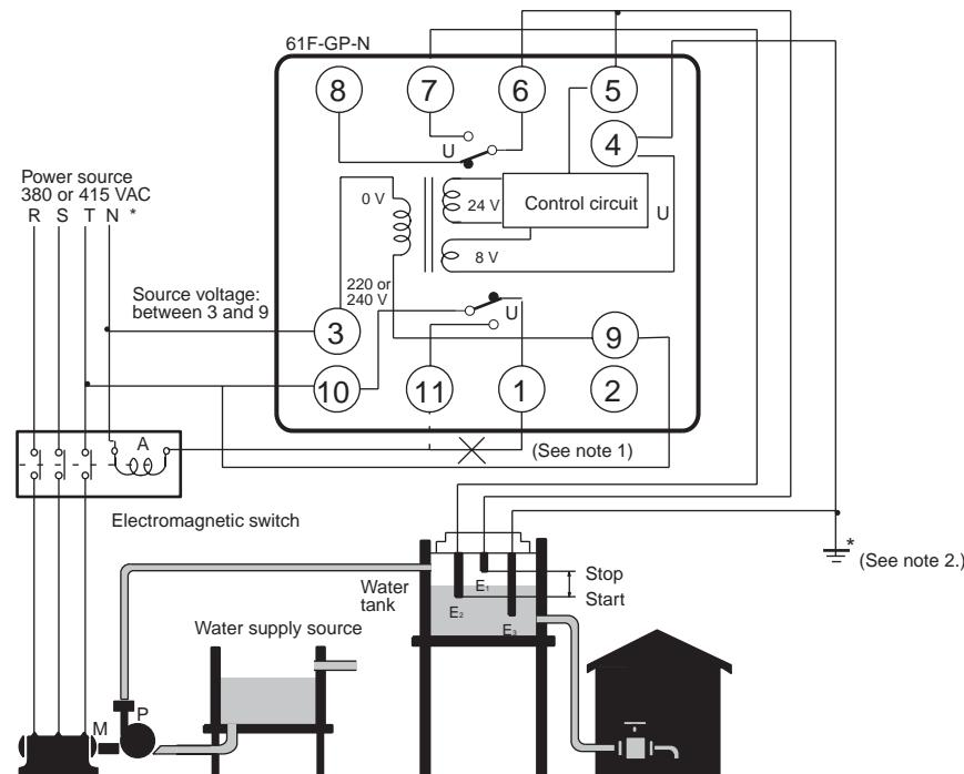
**Note:** 1. The diagram shows the connections for the water supply. When draining, change the connection from terminal 1 to terminal 11.
