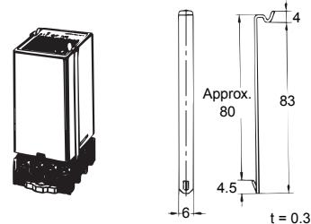
**Note:** PFC-N8 Mounting Bracket (provided with the Level Controller)
