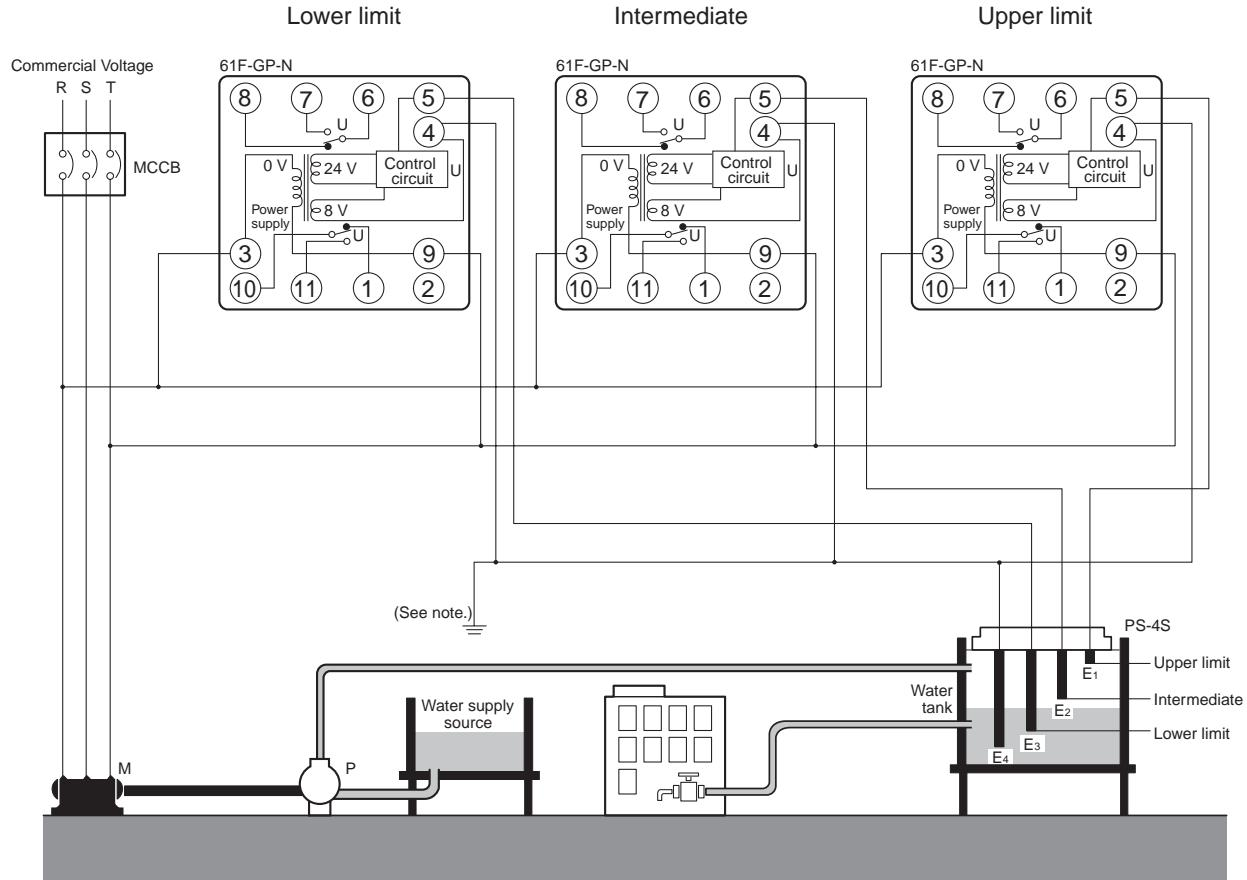
**Note:** The power supply phases (terminals 3 to 9) can be matched to use the same ground for the common Electrode (the longest Electrode, terminal 4).
