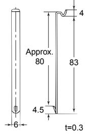
**Note:** PFC-N8 Mounting Bracket (provided with the Level Controller)
