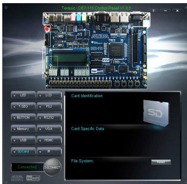
Figure 3-10 Reading the SD Card Identification and Specification
