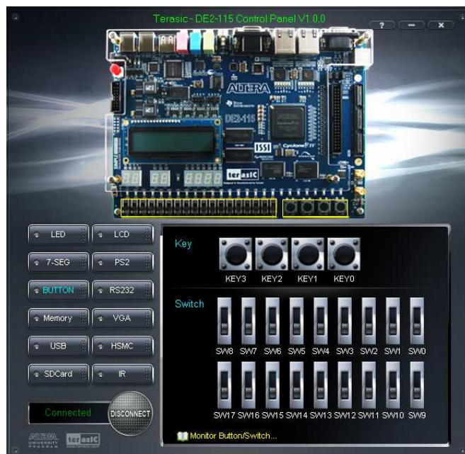
Figure 3-6 Monitoring switches and buttons
