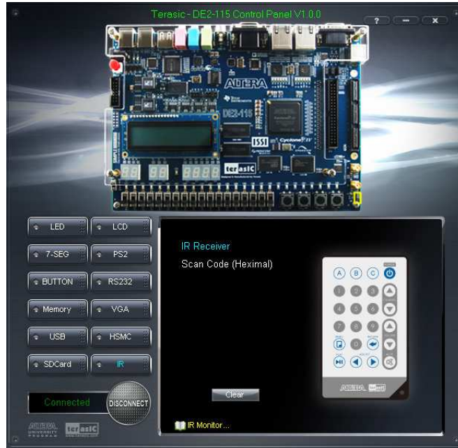
Figure 3-14 Testing the IR receiver using remote controller
