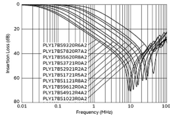
Differential Mode Insertion Loss-Frequency Characteristics
