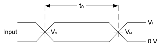
Voltage Waveform Pulse Duration
