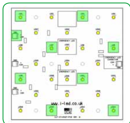
LEDs connected to CON4 - Emergency
