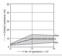
5-(2). Electrical life test (at capacitor load)
