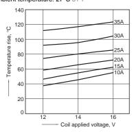
1-(2). Coil temperature rise Sample: CP1H-12V, 3pcs Point measured : Inside the coil Ambient temperature: 85°C 185°F
