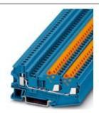
Feed-through terminal block, Connection type: Quick connection, Screw connection, Cross section: 0.5 mm² - 2.5 mm², AWG :20- 14, Width: 6.2 mm, Color: blue, Mounting: NS 35/7,5, NS 35/15
