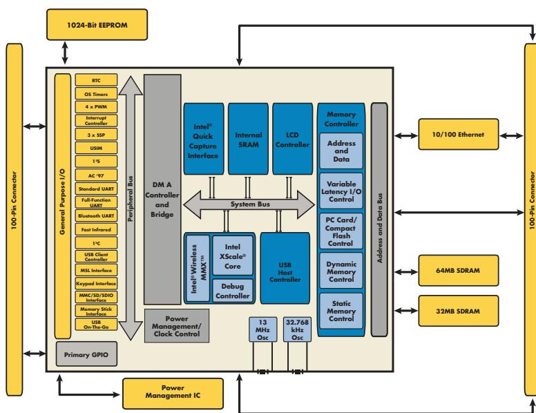
High-performance core module with Intel XScale processor provides complete embedded platform support, combining industry-leading performance, multimedia capabilities and low power requirements in an ultra-compact form factor.
