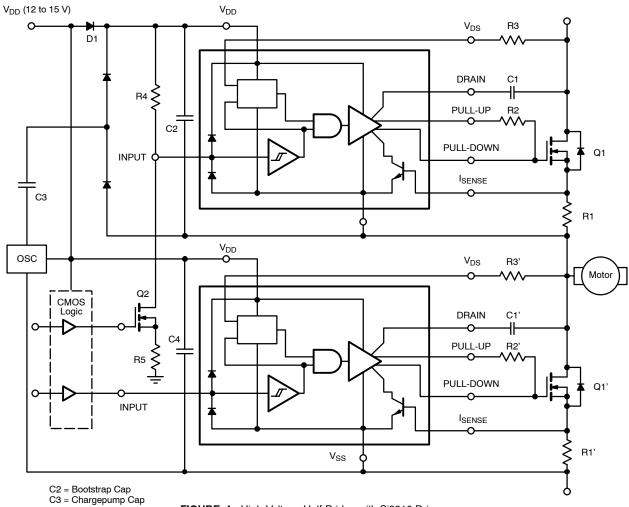
FIGURE 1. High-Voltage Half-Bridge with Si9910 Drivers
