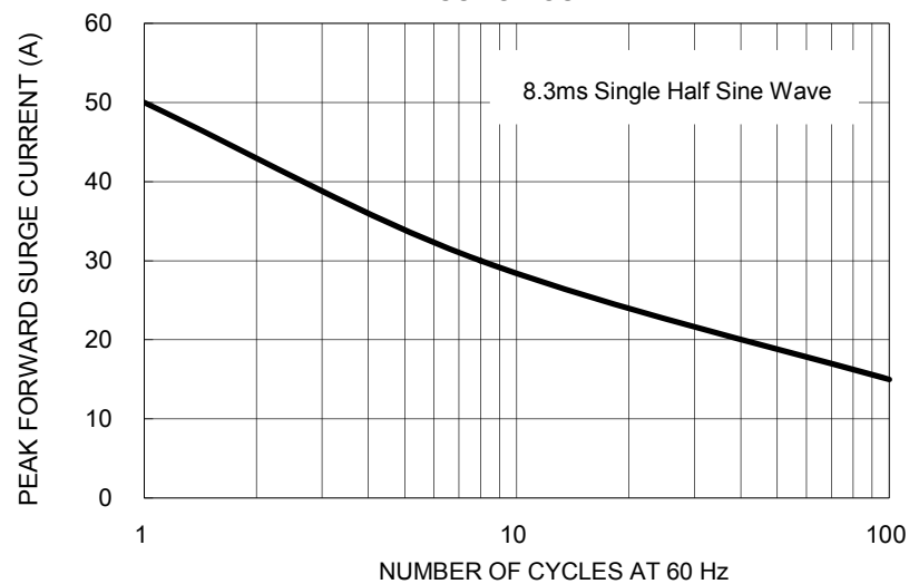
FIG. 3 MAXIMUM NON-REPETITIVE PEAK FORWARD SURGE CURRENT
