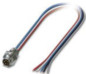
Bus system flush-type connector, plug, DeviceNet, 5-pos., M8, front/screw mounting with M8 fastening thread, with 0.5 m PVC litz wire, 5 x 0.25 mm 2
